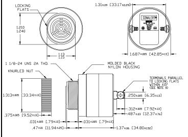
NOTE AF TERMINALS-032 BRASS TIN PLATED, TAPPED FOR #6-32 SCREW. TWO #6-32 NICKEL PLATED BRASS SCREWS INCLUBED. WILL ACCEPT 1/4' QUICK CONNECT. NOTE B: MOUNTING- REMOVE BLACK PLASTIC NUT AND INSERT THREADED FRONT THROUGH 1.25' HOLE PUNCHED IN PANEL, IF DRIENTATION IS NEEDED, NOTE LOCKING FLATS ON DRAVING. SCREW NUT BACK ON. DO NOT OVERTIGHTEN.
