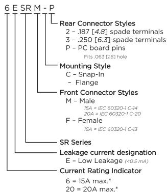
\*15A versions are tested by Underwriters Laboratories to US and Canadian requirements and are VDE approved at 10A, 250VAC 20A versions are tested by Underwriters Laboratories to US and Canadian requirements and are VDE approved at 16A, 250VAC
