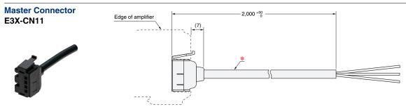
\* E3X-CN11: 4 dia. cable / 3 conductors / Standard length: 2 m (Conductor cross section: 0.2 mm² (AWG24), Insulator diameter: 1.1 mm)
