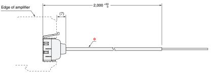
\* E3X-CN12: 2.6 dia. cable / 1 conductor / Standard length: 2 m (Conductor cross section: 0.2 mm<sup>2</sup> (AWG24), Insulator diameter: 1.1 mm)
