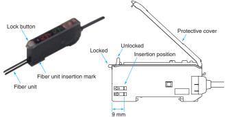
Note: If one of the fibers from the Fiber Unit is labeled as the Emitter fiber, such as with a Coaxial Sensor, insert that fiber into the Emitter section. Refer to *Dimensions for the Fiber Unit* to see if there is an Emitter fiber label.
