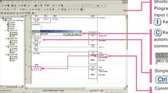
Shortcut keys can be easily checked using the ladder key guide.
