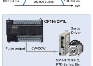
A positioning OMRON Function Block for the CP1H is used in the above application example. The positioning OMRON Function Blocks for the CP1L are the same as the positioning OMRON Function Blocks for the CJ1M-CPU21/22/23.
