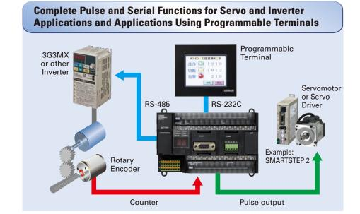
For positioning or communications, simply enter the set values for the instructions. Even complicated functions can be easily programmed using the OMRON Function Block (FB) Library.
