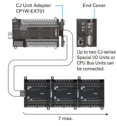
Use CP1W-CN811 I/O Connecting Cable when using CP1W/CPM1A Expansion Units and Expansion I/O Units at the same time as a CJ Unit Adapter. In this situation, the number of CP1W/CPM1A Expansion Unit and Expansion I/O Units that can be connected is subject to the restrictions described above. Only one I/O Connecting Cable can be used.
