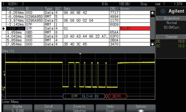
Figure 1: Hardware-based decoding quickly reveals serial communication errors.
