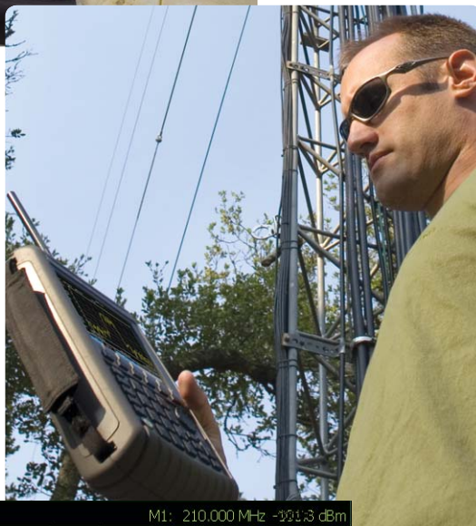
Use the spectrum analyzer's audio signal strength indicator to locate signals when walking around
