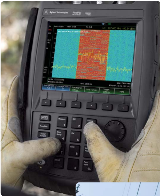
RF spectrum monitoring aided by spectrogram recording
