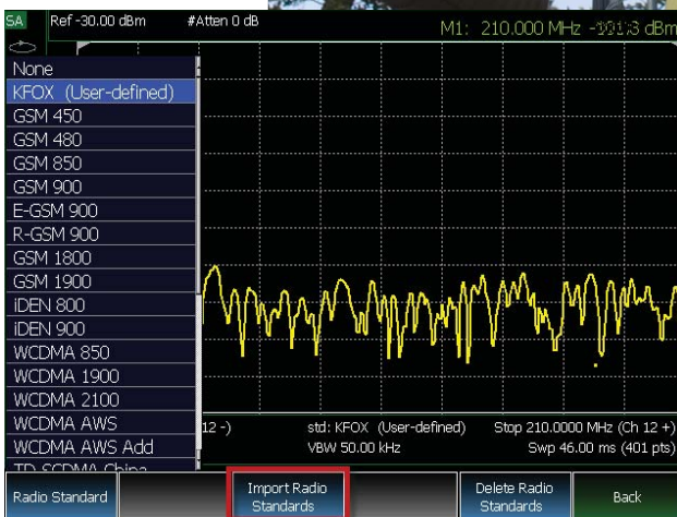
Select one of the pre-loaded radio frequency standards, or create your own custom standard
