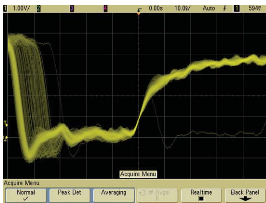
Figure 5. 256 levels of display intensity gradation show characteristics of jitter, noise, and signal anomalies.
