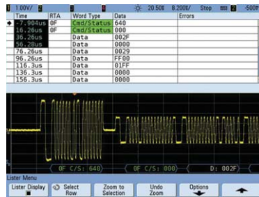
Time-correlated display of the MIL-STD 1553 physical layer signal with protocol decoding.
