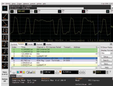
Trigger on and decode PCIe serial packets.
