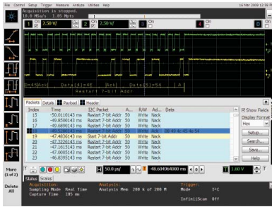
Trigger and view on-screen serial decode of I 2 C packets.
