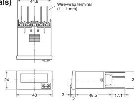
When using the Wire-wrap Terminal, be sure to use the correct wires and peripheral devices. (The correct wires, bits and sleeves are shown in the table on the right.)
