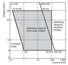
The above diagram is for standard conditions  $(+5^{\circ}C \text{ to } +35^{\circ}C, 40\% \text{ to } 70\% \text{RH})$ . Since the values vary depending on the operating environment conditions, contact your OMRON representative for further details.
