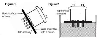
• Using a Soldering Iron
