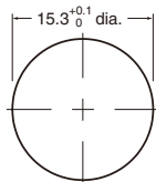
Panel Cutout Dimension Panel thickness = 1 to 4 mm
