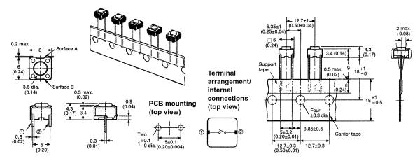
**Note:** The tape is random between surface A and surface B. Unit: mm (inch)
