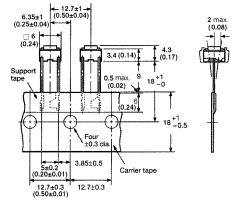
Note: The tape is random between surface A and surface B. Unit: mm (inch)
