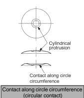
Switches have circular contact surface instead of single center point contact, increasing contact reliability.
