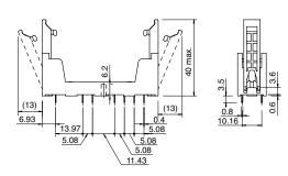
PC Board Mounting Hole Layout / Terminal Arrangement (Bottom View)
