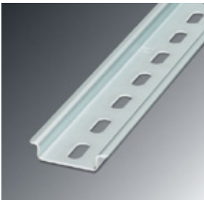
DIN rail perforated, Width: 35 mm, Height: 7.5 mm, Length: 2000 mm, Color: aluminum
