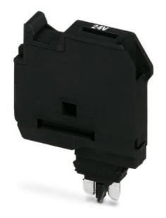
Fuse plug, black, with light indicator, voltage light indicator: 110 V ... 250 V, current light indicator: 0.5 mA ... 2.5 mA, color: Black
