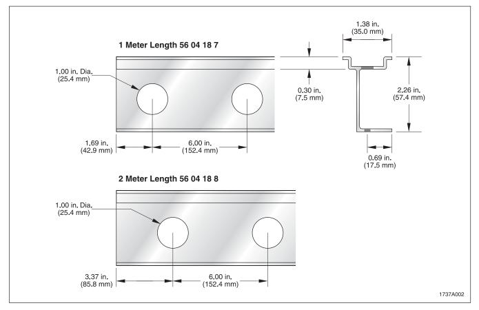
Figure 2. Perforated Aluminum Raised Rail Dimensions
