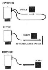
Fiber optic sensing is often the answer when, due to space or environmental limitations, the sensor itself cannot be placed at the actual sensing position. These sensors' powerful modulated infrared beam is compatible with all Banner glass fiber optics in the opposed, retroreflective, and diffuse sensing modes. See Banner catalog for glass fiber optic selection information . Sensor/fiber interface is waterproof to maintain complete sensing system moisture rejection.
