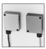
**Range:** 50 feet (15m) Effective Beam: .5 inch (13mm) dia. Temp. range: -40 to +100 degrees C Housing material: anodized aluminum
