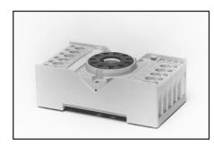
The RS-11 is supplied with a coding ring and pin (see diagram at right). This allows a MAXI-AMP to be keyed to fit only its own 11-pin socket. The pin is installed in one of the eleven slots in the RS-11, and the notch in the ring is aligned to slip over the pin. When the MAXI-AMP is removed from the RS-11, the coding ring stays with the MAXI-AMP base, while the coding pin remains in the socket.
