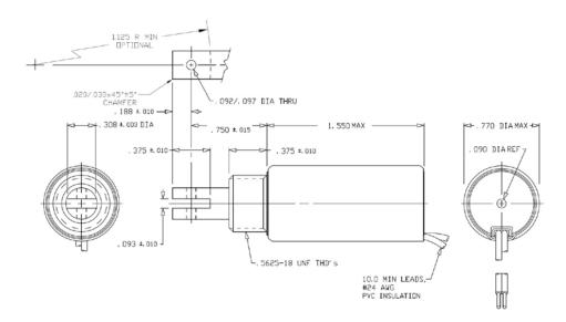
Solenoid shown energized with plunger fully seated Supplied with hex nut shipped loose Spring kits available (consult factory)
