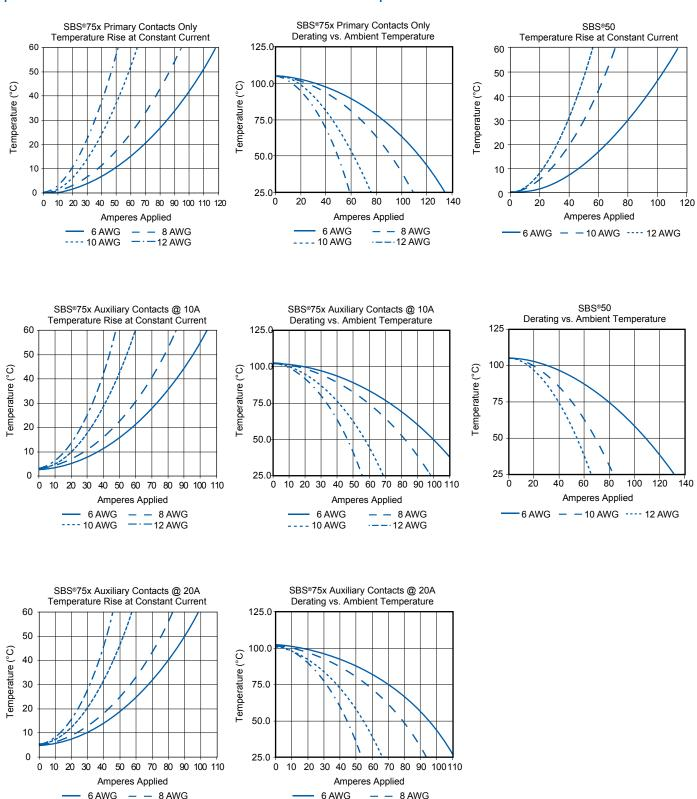
NOTE: Temperature rise charts are based on a 25°C ambient temperature.
