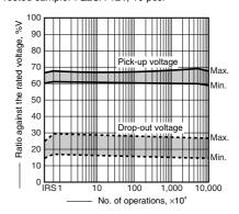
4.-(1) Electrical life (2 A 30 V DC resistive load) Tested sample: TQ2SA-12V, 6 pcs.
