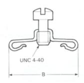
For steel screw lock assemblies the maximum recommended assembly torques are :
