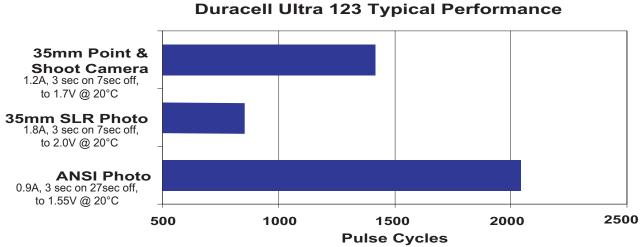
\* Delivered capacity is dependent on the applied load, operating temperature and cut-off voltage. Please refer to the charts and discharge data shown for examples of the energy / service life that the battery will provide for various load conditions.
