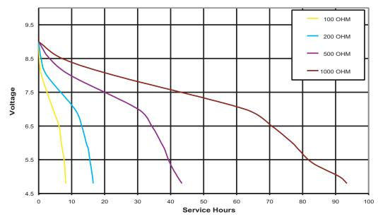
\* Delivered capacity is dependent on the applied load, operating temperature and cut-off voltage. Please refer to the charts and discharge data shown for examples of the energy / service life that the battery will provide for various load conditions.
