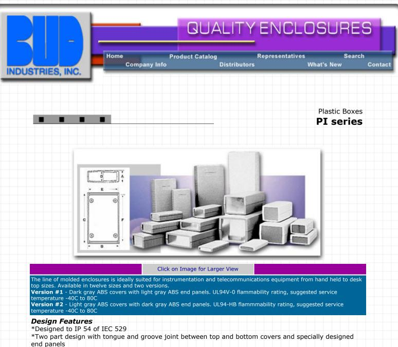
\*Internal guide slots provide for vertical mounting of PCBs
