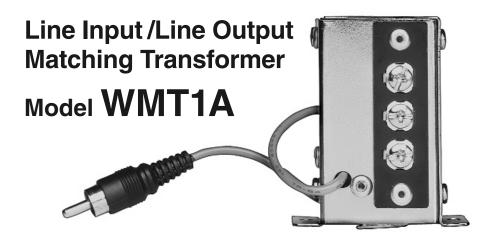
The **WMT1A** is a balanced and isolated impedance matching transformer. Typical uses are to provide a 600-ohm balanced input adapter for unbalanced AUX inputs. WMT1A can also be used to drive long, balanced, twisted pair cable. This improves noise rejection and the maximum run length. The WMT1A can adapt line-level signals down to levels suitable for MIC inputs. See the drawing below for setting the Operating Modes.
