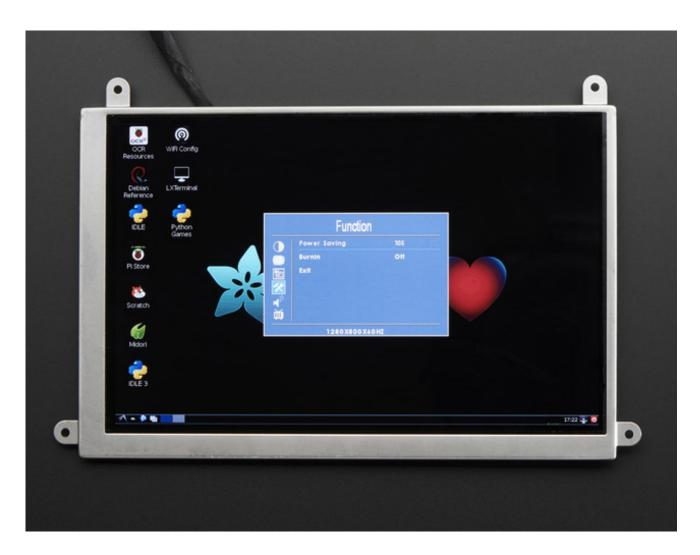
**Power Saving -** 10s to 60s - how long it takes for the screen to shut off **Burnin -** On/Off - a function to prevent screen burn-in (http://adafru.it/dTR)
