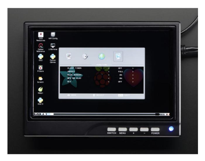
**Sleep Timer** - to 120 minutes - this will completely shut off the screen at the end of the set time **Aspect** - Full
