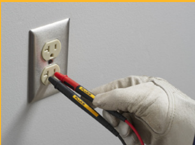
Extend tip for CAT II probing
