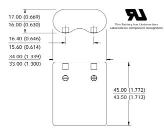
This battery contains a Positive Temperature Coefficient (PTC) safety device to limit current during short circuit conditions.
