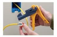
Release handle and remove jack from JackRapid tool. Visually verify proper termination.
