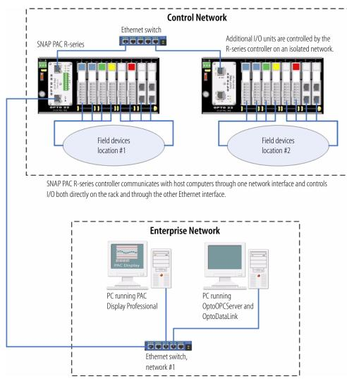
This diagram shows two SNAP PAC I/O units connected together over an Ethernet network and controlled by a SNAP PAC R-series controller running a PAC Control strategy.
