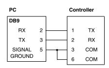
\* Minimum requirements for wiring an RS-232 serial cable to connect to a PC. If you want to connect the controller to a modem, see form #1595, the SNAP PAC R-Series Controllers User's Guide, for all eight pin connections.
