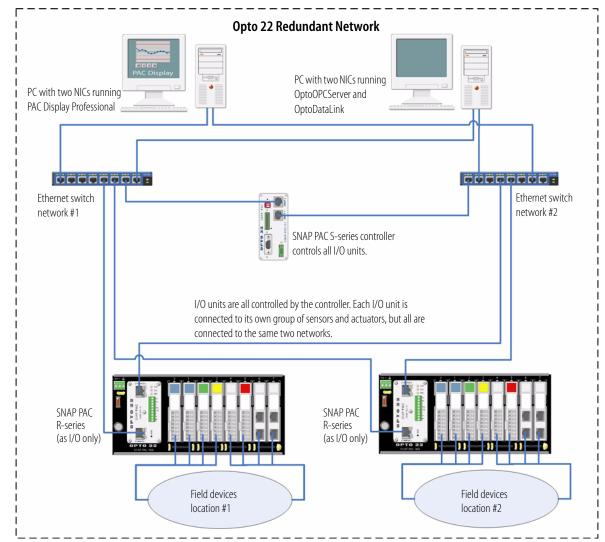
This diagram shows two SNAP PAC R-Series controllers functioning as I/O unit brains connected to two separate Ethernet networks. This configuration addresses the concern that an Ethernet network may fail or need maintenance, leaving the PC running OptoOPCServer and OptoDataLink, the PC running PAC Display, the controller, and the I/O units unable to communicate.
