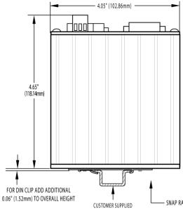
35mm DIN RAIL NOTE: BESURE TO CONSIDER DIN RAIL DIMENSIONS.
