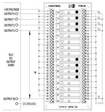
$<sup>^{\</sup>star}$  This wiring can be done using a G4STRAP.
