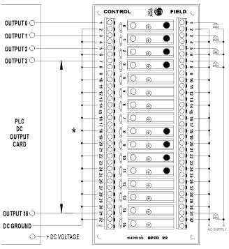
$<sup>^{\</sup>star}$  This wiring can be done using a G4STRAP.
