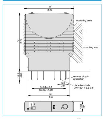
This is a metric design and millimeter dimensions take precedence ( $\frac{mm}{inch}$ )
