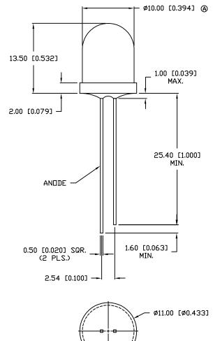
UNLESS OTHERWISE SPECIFIED TOLERANCE IS ±.25mm (±0.010")
