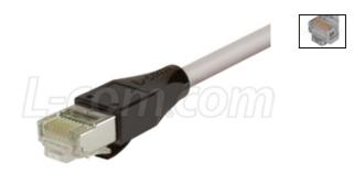
For maximum protection against EMI/RFI interference, L-com's Double Shielded Patch cables are the right choice. With two layers of shielding (Foil plus Braid), data is protected from stray EMI/RFI fields. This series features 24AWG solid conductors allowing easy termination to IDC connectors. The rugged LSZH jacket is extra durable for harsh industrial environments. L-com stocks lengths up to 300 ft and can ship most orders the same day.
