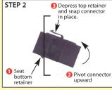
Seat bottom retainer and pivot connector upward while depressing upper retainer
