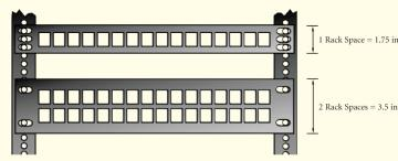
Racks are a great way to neaten up wiring closets and labs. Network equipment and rack panels usually come in 1.75", 3.5" and 5.25" heights. (1, 2 and 3 rack spaces).
