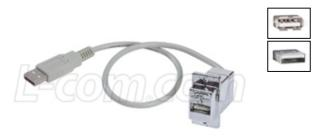
Another unique panel mount USB option features a bulkhead Type A jack to a molded Type A plug with 12" of USB 2.0 compliant cable. The 12" cable can be directly connected to a mating connector inside an enclosure. This assembly is fully shielded, 12 inches long, and uses the popular ECF style housing that is usable in virtually any panel thickness. Recommended 4-40 mounting screws must be purchased separately (P/N ECF440).
