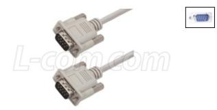
L-com's top of the line offering of D-sub cable assemblies provide maximum protection against data corrupting EMI/RFI. Double shielded cable (copper braid plus aluminum mylar foil) and a custom steel internal enclosure separate these cables from any off the shelf D-sub cable on the market. Ideal for any electrically noisy environment where fans, motors or switches are nearby. Custom lengths and pinouts are available with modest minimum requirements.
