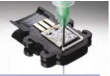
dispensing to auto-dispensing units for tube, cartridge, pail, or drum packages. Mixing for 2 Part grades may be accomplished by either manual processes or meter mix dispensing, depending on production volume and post-mix material properties.
