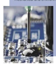
are offered in various cure speeds. viscosities, and performance, many of which offer enhancements for thermal cycling protection, stress relief, material strength, flame retardancy, or optical clarity.
