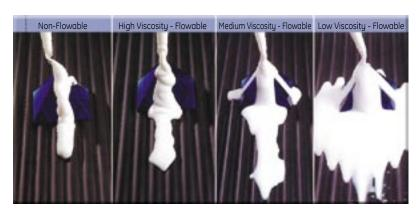
Viscosity and flowability of the silicone material are often key factors in the selection of a material for use in sealing, coating, and encapsulation / potting applications. A broad array of material performance and viscosity combinations are provided to help match the requirements of many applications.
