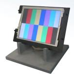
6.4" display, resistive touch screen, high bright, sunlight readable, moisture sealed transportation communication panel, ruggedized to SAE specifications
