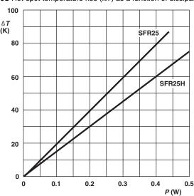
**SFR25/SFR25H** Hot-spot temperature rise ( $\Delta T$ ) as a function of dissipated power
