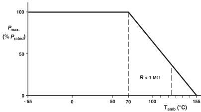
Maximum dissipation ( $P_{\text{max}}$ ) in percentage of rated power as a function of the ambient temperature ( $T_{\text{amb}}$ ).
