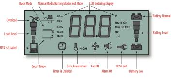
All SLF Series UPS are equipped with a convenient front panel LCD status display. This provides immediate UPS and site power status without the need for externallyconnected computers or workstations. Over twenty UPS statuses and conditions can be displayed.
