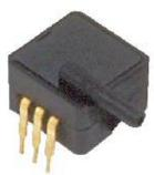
Pressure Sensors: Measurement Type: Absolute; 0 psia to 15 psia, Temperature Compensated Sensor, "A4" Package - Straight Port
