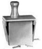
Snap-in Panel Mount Switch, Single Pole Double Throw (SPDT) Circuitry, 10 A at 277 Vac, Finger Grip Plunger Actuator, Silver Contacts, Quick Connect Termination
