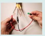
GREEN LED means wiring is properly identified.
